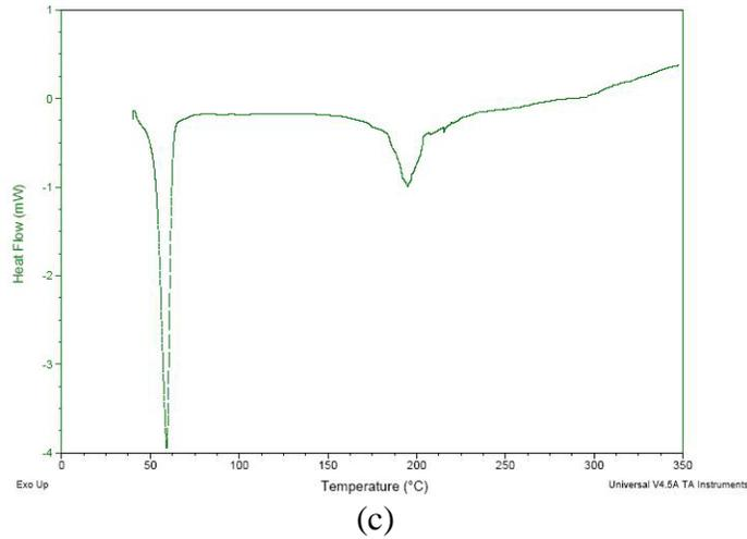
Figure 3: DSC thermograms of (a) bulk lipid (b) compound (c) compound loaded SLN
