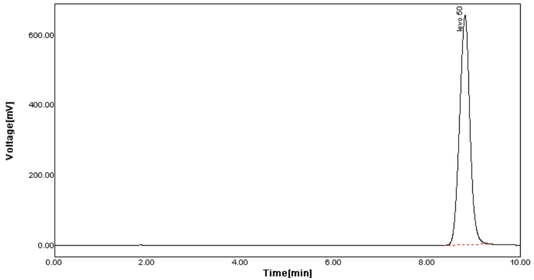
Figure: 1 Atypical chromatogram for levofloxacin solution (50µg/ml)
