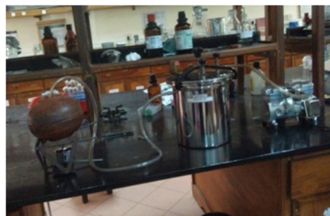
Figure 4: Fumigation Apparatus (Mud Pot, McIntosh jar & Vacuum pump)
