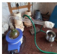
Figure 18: Preparation of Arka using simple distillation
