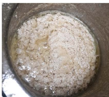
Figure 17: Oil completely separated after reheating
