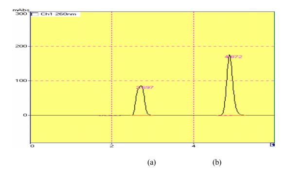
Fig 2: Typical chromatogram showing the elution of (a) Torsemide (20µg/ml) and (b) Spironolactone (50µg/ml) at their respective retention times
